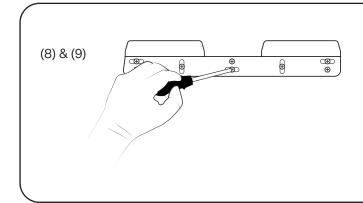
8) Use the 2 x Hex Head Screws (M5) for the center holes, which are in-line with the stud, to fix the cleat to the wall.
