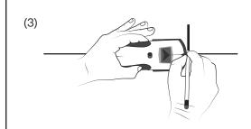
3) Along the line you just made, find a wall stud. Mark the stud's location underneath the line you drew. When installing your Alter Screen into drywall, the wall mounting cleat must be connected to a stud. If you cannot find a stud, or don't have a stud finder tool, purchase one at any local hardware store.
