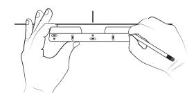
4) Place the wall mounting cleat in a position where it is both level and in-line with the stud you've marked. The top of the wall mounting cleat should be below the horizontal line you've drawn, just enough to still see the line slightly above the top edge of the cleat.
